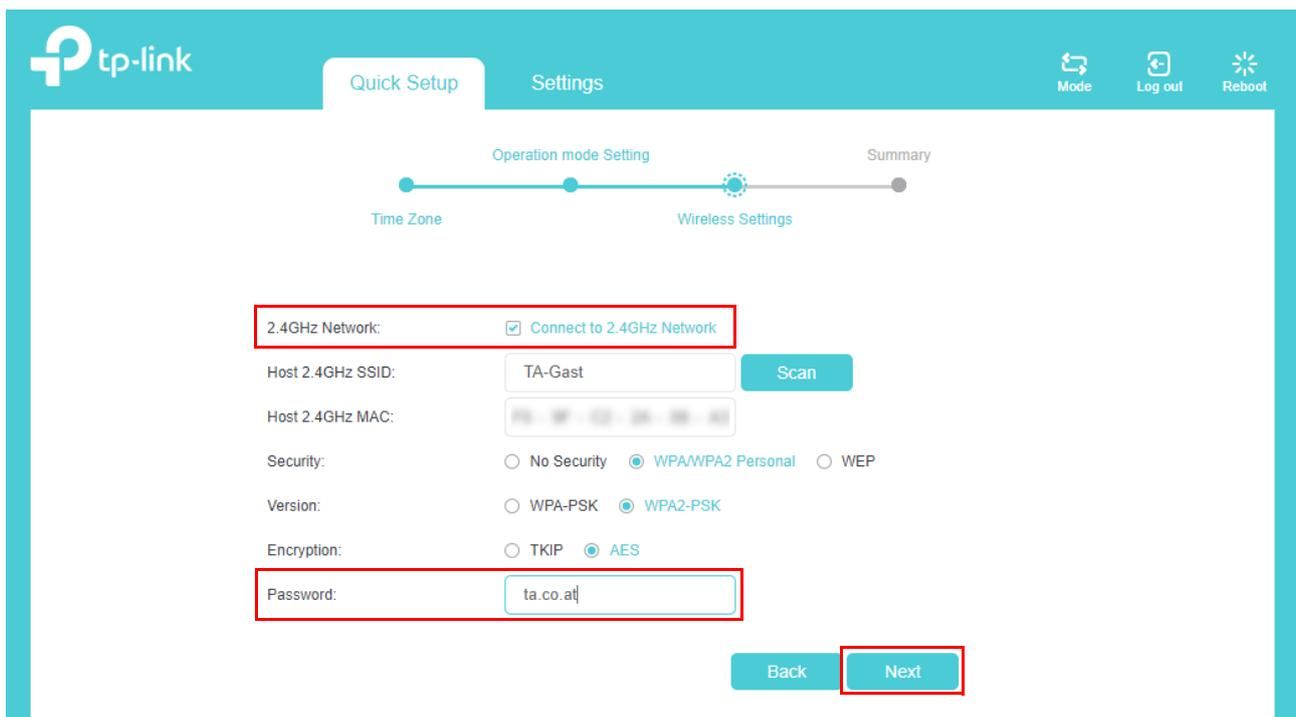
The screenshot shows the 'Wireless Settings' step in the TP-Link Quick Setup wizard. The '2.4GHz Network' checkbox is checked. The 'Next' button is highlighted in red.
