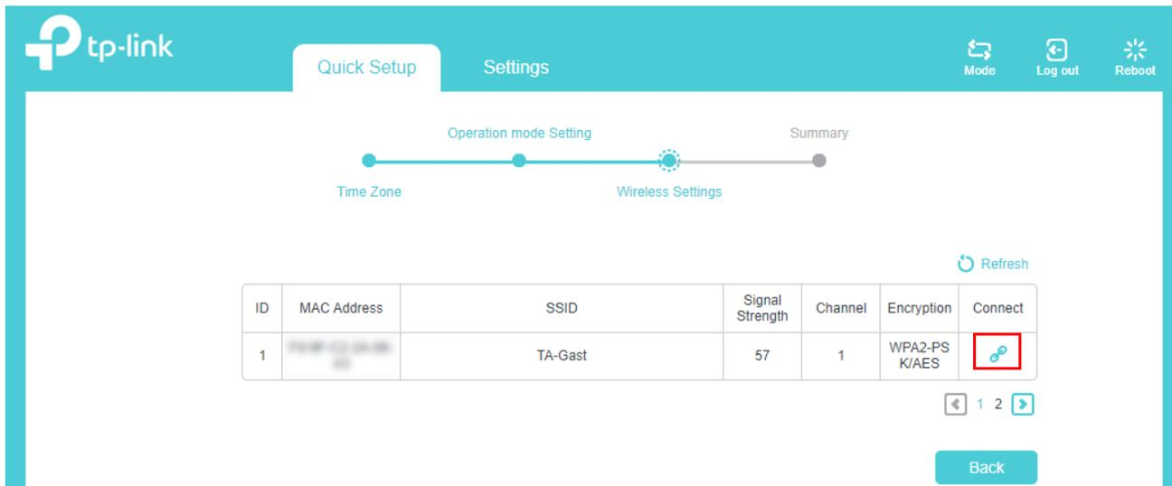
The screenshot shows the 'Wireless Settings' step in the TP-Link Quick Setup wizard. A progress bar at the top indicates the current step. Below it, a table lists available networks. The 'Connect' button for the selected network is highlighted in red.
