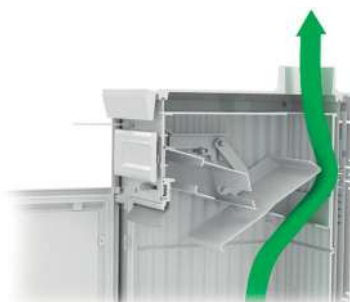
SMOKE BY-PASS ON
